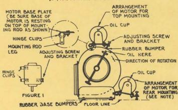
NOTE: Figure 1 is for top mounting only. For rear mounting, bolt hinge clips and adjusting screw and bracket opposite to the way shown.
